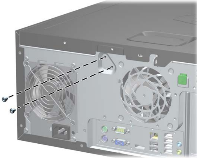
Figure C-1 Removing the Smart Cover Lock Screws from the Convertible Minitower
